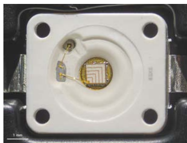
High brightness LED, chip, bond wires and packaging, OL, Spot K LED, 1.25x
